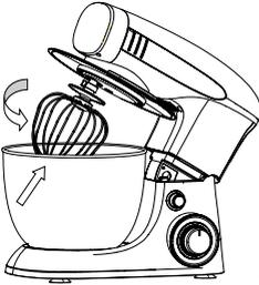
7. Fit the required accessory (11 with 10, 9) onto the motor spindle (7) on the underside of the swivel arm (2).
