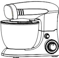
10. Lower the swivel arm so that it locks into place. The bowl cover (8) must fit tightly with the mixing bowl (13), otherwise it is fitted incorrectly. The appliance is now ready for use.
