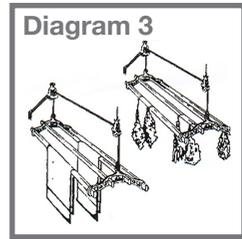
10. Pull up the airer until the airer is at the required drying height close to the pulleys. Tie another knot in the two cords at the point it is with the cleat. This is so you can hook the rope on the cleat to hold your airer up in the air while your clothes are drying. Your airer is now operational and will give you many years of problem free use.
