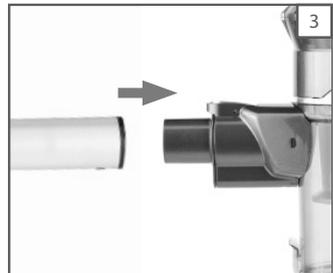
4. Connect the telescopic extension tube (6) into the brush head (7) (Fig 4).
