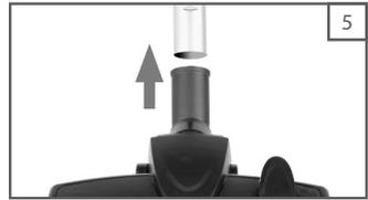
2. Remove the telescopic extension tube (6) from the accessory adapter (10) (Fig 6).
